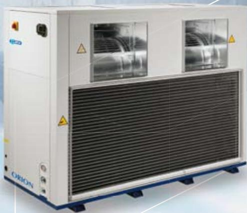
The ORION range of chillers and reversible heat pumps, featuring centrifugal fans, offer either single or, above 50 kW, tandem scroll compressors. Plate heat exchangers are applied and the pump and buffer tank are included within the package, to the benefit of installation and start-up.
